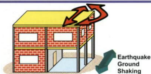
Figure 5: One-side open ground storey building twists during earthquake shaking.
